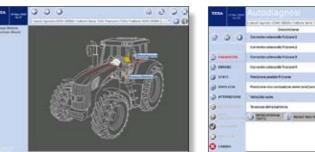
selecting make, model and engine type, IDC3 Agri allows you to access all the active functions for that particular vehicle.
