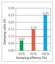
Damping ratios  $\vartheta$  determined with suspension tester contactest 3800 on shock absorbers having different damping efficiencies; the ratios were determined on a car under in-situ conditions.
