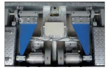
The vibrating mass-spring-system of the test stand is specially adjusted to the resonance vibrations of vehicle suspension. Consequently the damping ratio according to Lehr is determined without any interferences from the test stand.
