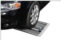
As the lifting device raises the vehicle to ground level, driving in and off the rollers is considerably facilitated and hence especially advantageous for vehicles with sports chassis, low ground clearance or small wheel diameters in that it minimises the risk of underbody damage.
