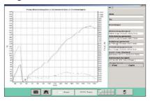
In this program power and torque are determined. The car is accelerated from standstill to maximum speed by changing gears smoothly but quickly. Once the level of maximum power has been exceeded, the clutch is disengaged and the car is allowed to coast. During coasting power loss is constantly determined. After coasting the measured values of power, velocity and torque are read out both in form numerical values and graphically.
