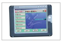
Mobile monitor for transmission of measured data and other information. The entire test sequence is conveniently controlled from driver's seat.
