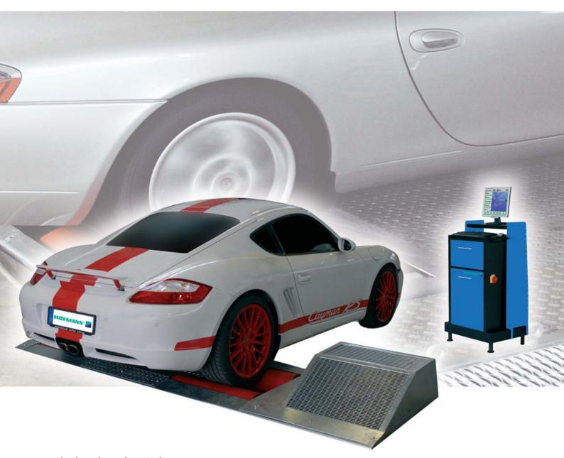
Single-axle and 4WD dynamometers
