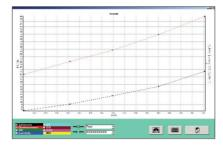
In this program a velocity can be preset for the car under test in order to simulate various loads. The velocity can be changed during the test so that the behaviour of the car can be tested at different velocities. Upon completion of the test the values measured at the preset velocities are read out.
