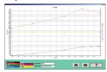
This program is designed to simulate loads. To this end a predefined force is set for the car under test (uphill driving). The load can be varied during the test. Upon completion of the test the values measured at preset loads
