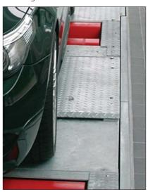
A hydraulic displacement mechanism, which is used for adjustment to the vehicle's wheelbase, is controlled with the infrared remote control.
