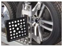
Once the four targets are fitted on the wheels, the complete alignment readings are available within seconds. This allows to carry out more alignments a day - and your investment pays off within short.
