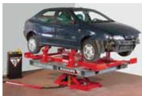
The vehicle comes down to rest on the underbody clamps.
