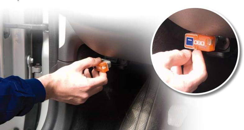
OBD Log is a sophisticated diagnostic device that plugs directly into a vehicle's OBD socket without impeding normal vehicle use in any way.
