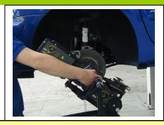
2. Connect the lathe and machine the disc (6 Mins)
