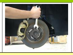
1. Remove the wheel and fit adaptor (3 Mins)
