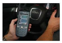
The optional PWA (pocket workshop assistant) is a pocket PC with Hofmann testing software and integrated remote control which can replace other display units such as display cabinet or monitor. The entire test sequence is controlled from driver's seat. Only the function keys required for the current test are displayed on the screen. Control is via touch screen. A PC station is necessary for connection of the PWA.
