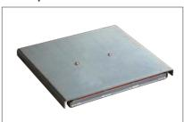
The side-slip tester is designed to measure toe of the vehicle under test immediately. No additional tests are necessary as the testing plate is positioned directly in front of the suspension tester and the vehicle simply rolls over. The data automatically detected supplies a sound diagnostics of toe-in and toe-out. The measured value is read out in 0 +/- 20 mm/m.
