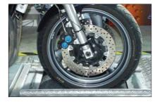
Car brake testers and test lanes can be easily retrofitted for motorcycle tests.
