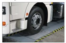
The side-slip tester is designed to measure toe of the vehicle under test. The results of toe-in and toe-out respectively are read out on the optional integrated LED on the display cabinet, or in graphical form on the optional monitor.
