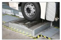
The lifting device HBV 4000 can be used only in conjunction with safelane truck N 20t with wheel / axle load weighing unit to simulate various wheel / axle loads. The roller set is raised and pressed against the vehicle under test.
