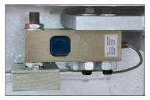
The wheel / axle load weighing unit is designed to automatically detect, calculate and store weight. The values are read out on the optional integrated LED on the display cabinet, or in graphical form on the optional monitor.
