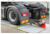
The joint play detector is a useful supplement for check-in or inspections to carry out a visual check of axle play. The galvanised test plates are operated hydraulically upon key operation of the test lamp. The test plates can be controlled one by one, in counterdirections (4-way control), or in same directions (8-way control).
