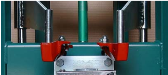
Low lips jaws for most vehicles manufactured in Japan
