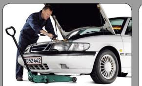
Ideal for support of engine/ transmission components during repair, with vehicle in low height.
