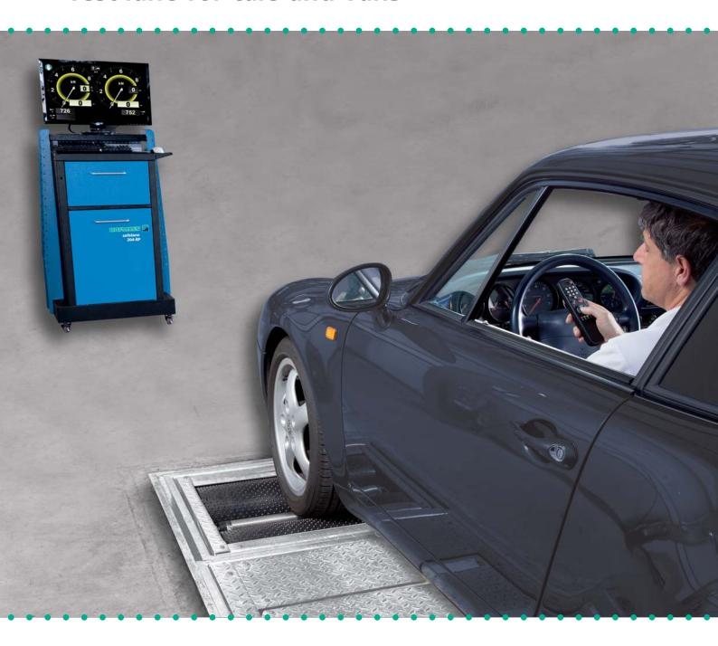
Modular system upgradeable into test lane
