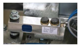
The features to be tested are detected by means of well-proven strain-gauge type load cells. This wear-free measuring system ensures reliable and error-free measurement of the forces produced.
