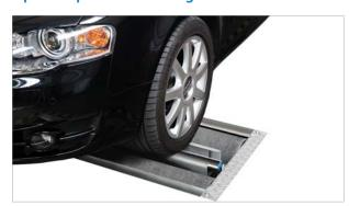
As the lifting device raises the vehicle to ground level, driving in and off the rollers is considerably facilitated and hence especially advantageous for vehicles with sports chassis, low ground clearance, or small wheel diameters where damage to the underbody is very likely under usual conditions.
