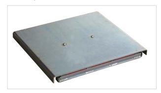
The side-slip tester is designed to measure toe of the vehicle under test immediately. No additional tests are necessary as the testing plate is positioned directly in front of the suspension or brake tester and the vehicle simply rolls over. The data automatically detected supplies a sound diagnostics of toe-in and toe-out. The measured value is read out in 0 +/- 20 mm/m.
