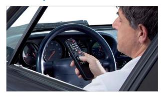
The optional radio remote control unit can be used to control the testing equipment from driver's seat at the entire discretion of the operator, e.g. by starting the brake tester only, or by conducting the tests in the sequence he prefers.
