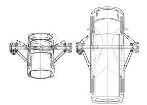
Thanks to the **Versymmetric® Technology** vehicles with short (i.e. Smart) as well as long wheel base (i.e. VW T5 long) can be lifted comfortably
